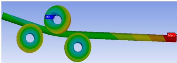
Figure 3: Simulation of pipe bending process.
