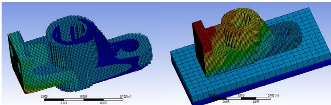
Figure 4: Additive manufacturing of a 3D product in Ansys.
