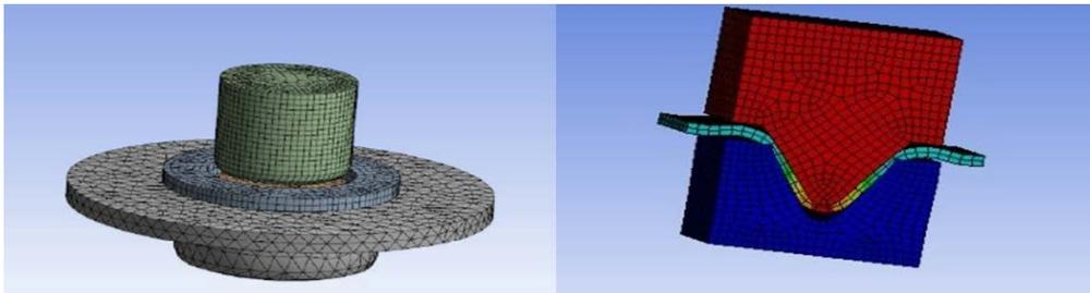
Figure 2: Metal deep drawing process simulations in Ansys.
